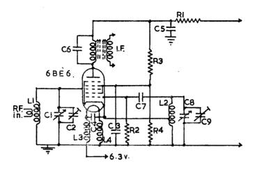
LI, L2, 13/4 turns 16 SWG, tinned copper Dia. 3/4, spacing between turns 3/8. Position of cathode tap on L2 is dependent on circuit layout.
